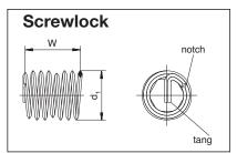
W and  $d_1$  are the control values for thread inserts (Free Running and Screwlock) before they have been installed. The length can only be measured for installed thread inserts.
