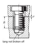
Prior to tapping, counter-bore 90° and deburr. Outside diameter of **countersink** =  $D_{HC}$  + **0.1** mm.
