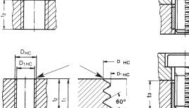
Prior to tapping, counter-bore 90° and deburr. Outside diameter of **countersink** =  $D_{HC}$  + 0.1 mm.
