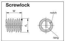
W and d<sub>1</sub> are the control values for thread inserts (Free Running and Screwlock) before they have been installed. The length can only be measured for installed thread inserts.
